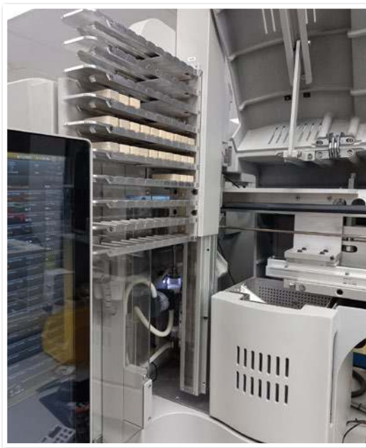
Crucibles containing wheat flour samples awaiting analysis for the determination of the nitrogen content. The nitrogen content is converted to crude protein content by multiplication with a factor of 5,7.
