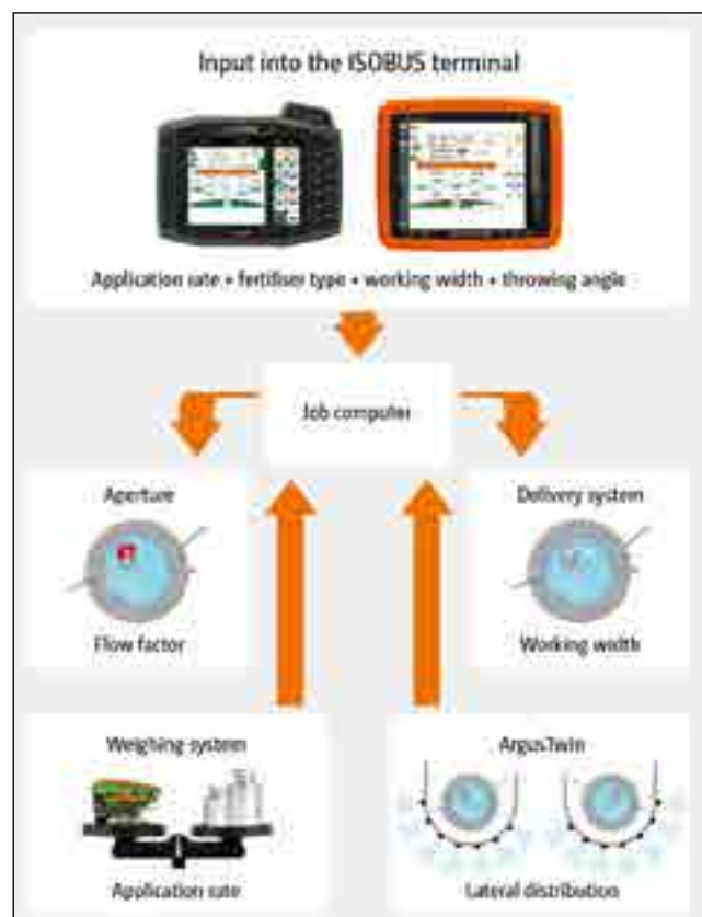
Figure 1: Radar sensors monitor both the left and the right spread-fans. As required, the lateral distribution is automatically optimised through the delivery system.
