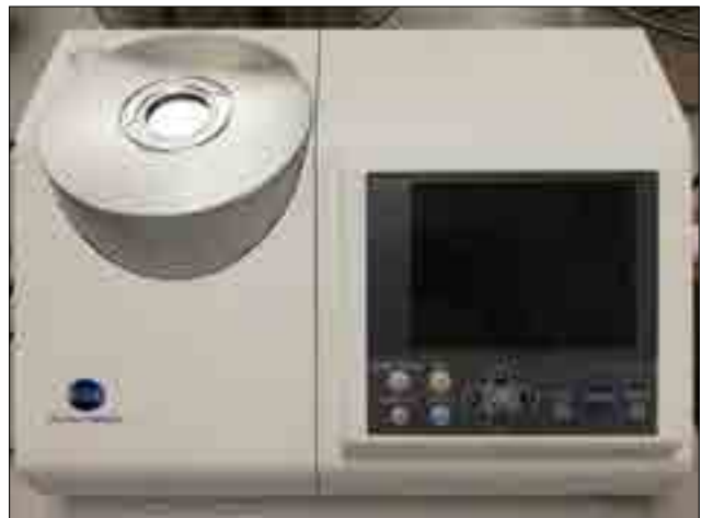
The Konica Minolta CM-5 spectrophotometer used to measure flour colour. The model uses lightness (L*) and two colour values (a* and b*). Generally speaking, a bright white colour flour is more desirable for most products.
