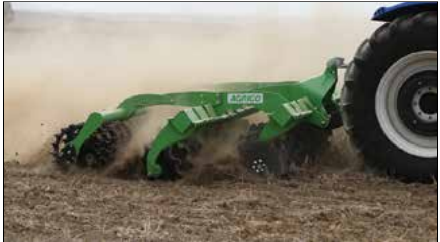
Die Agrico HSD 630 in aksie, besig om koringstoppels in te sny – vinniger as 14 km/h.
